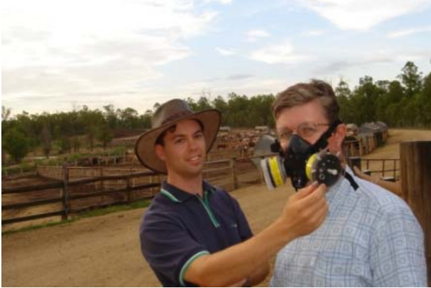
Chris giving a lesson on using a field olfactometer.
