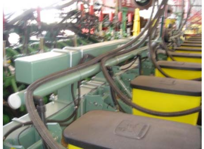
Australian made planter toolbar (3-pt), note use of US made John Deere row units.
